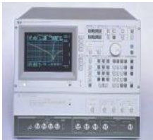
4194A ZA / Gain-Phase 100 Hz to 40 MHz (ZA) 10 Hz to 100 MHz (G-P)
