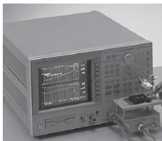
4395A NA/ZA/SA 100 k to 500 M (ZA) 10 Hz to 500 MHz (NA)
